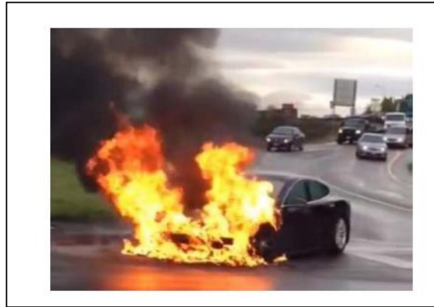
Fig. 4 Tesla S vehicle on fire as a result of battery penetration and a short circuit.
