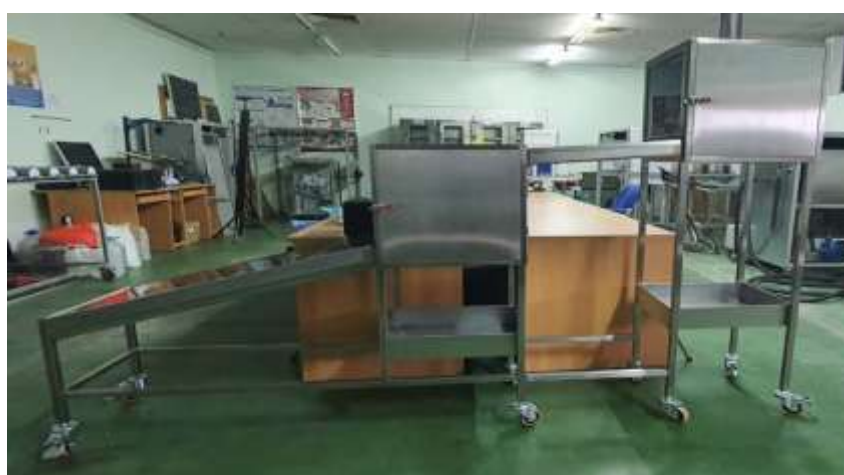
Fig. 2 Photo of solar dryer system
