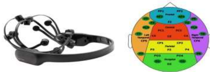
Fig. 2. Emotiv EPOC X mobile EEG headset and electrode placements, (Emotiv, 2025)
