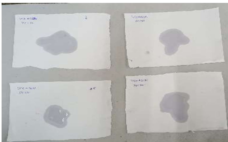
Fig: 1.7.1.d spread ability test for a. soyabean, b. sunflower, c. rice bran, d. groundnut oil
