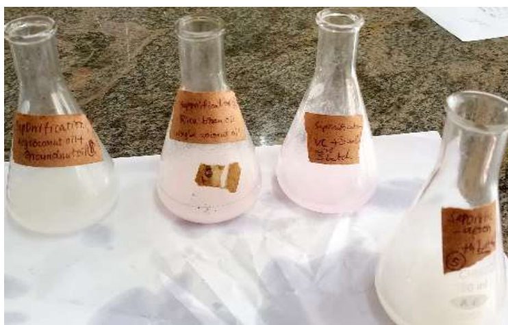
Fig: 1.7.3.2. Peroxide value test a. soyabean, b. sunflower, c. rice bran, d. groundnut oils
