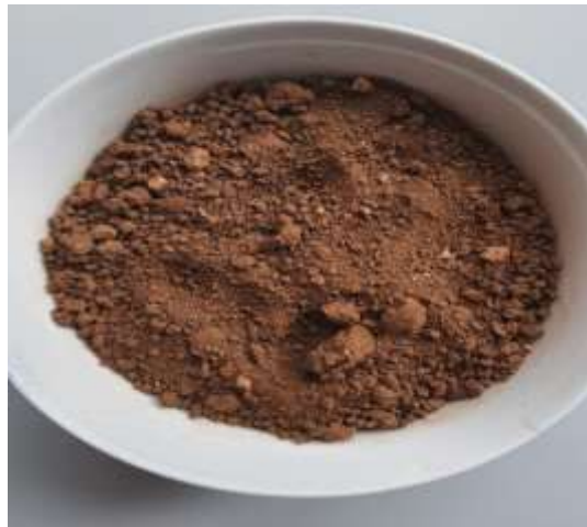
Figure 1. A-2-7 soil used in experiments, showing its untreated texture before stabilizer application.
