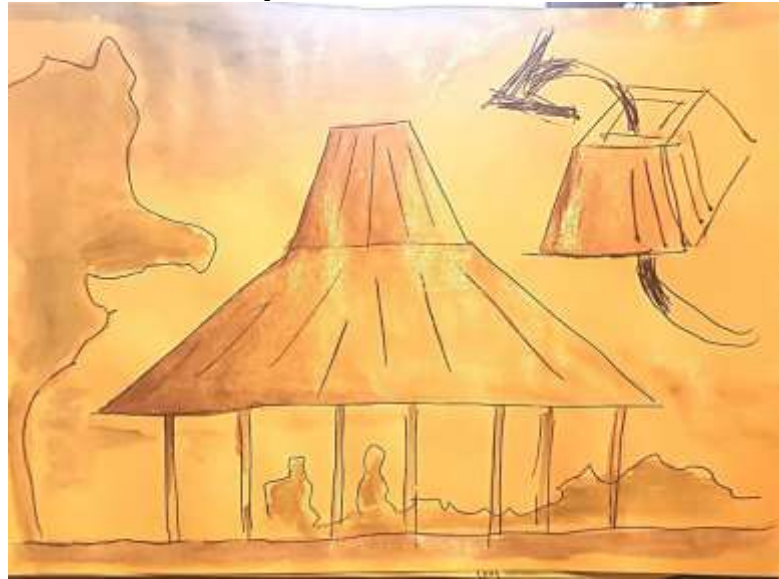
Fig. 3. Ventilated roof structure found in almost every building
