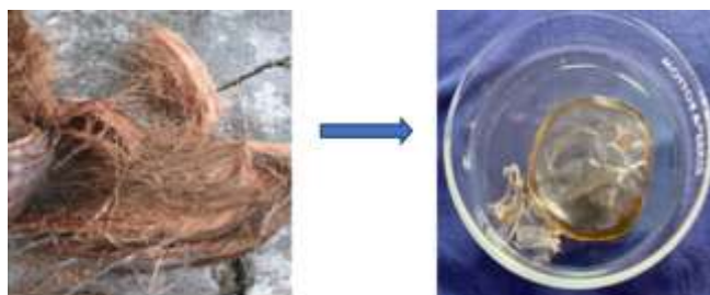
Fig. 6. Raw CC fiber converted into bioplastic film
