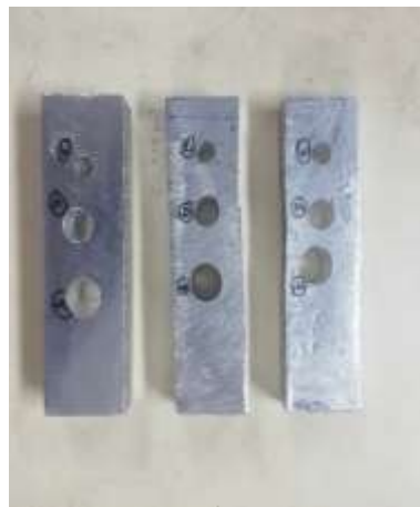
Fig. 1 Work Material (a) Developed MMC (b) Work Pieces before drilling (c) Work Pieces after drilling
