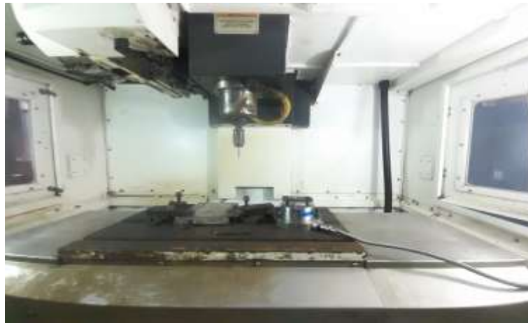
Fig. 3 Fitting the Workpiece and Drill Bit On VMC
