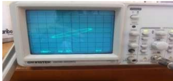
Fig. 12 photo of the Lissajous figure displayed on the oscilloscope when operating in the X-Y mode
