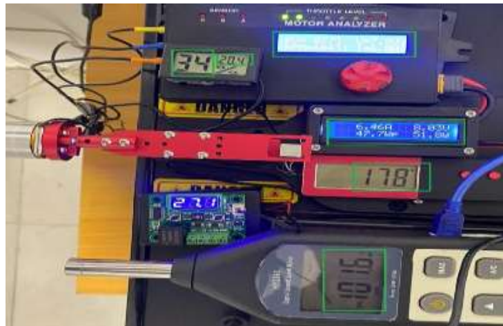
Fig. 4. Camera view showing OCR regions of interest for automated data extraction.
