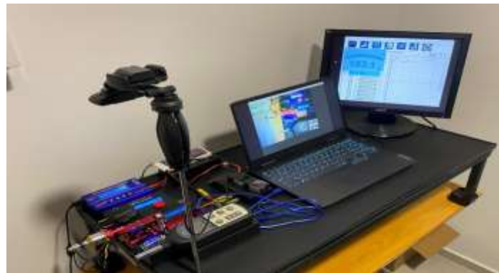
Fig. 3. Full experimental table showing motor, propeller, sensors, power distribution, laptop, and external monitor.
