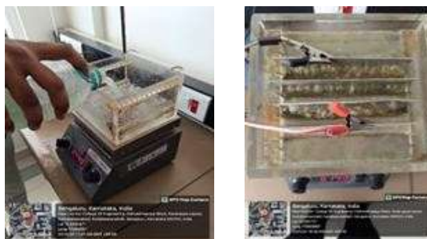
Figure 4 Setup Arrangement with Washing Machine Sample and Electrodes
