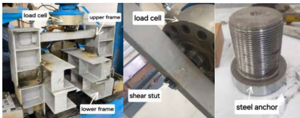
FIGURE 8. Details installing the metal frames.
