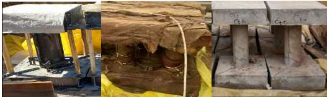
FIGURE 7. stages of curing concrete for the specimens.
