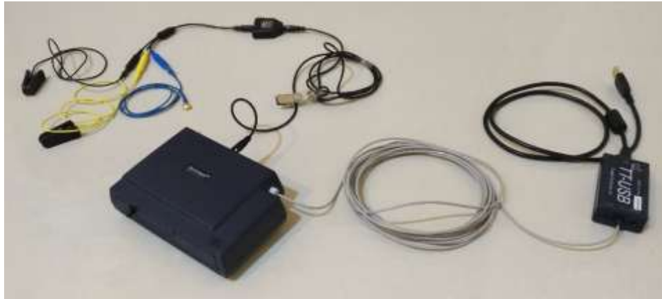
Fig.5 ProComp5 Infiniti device (Authors)
